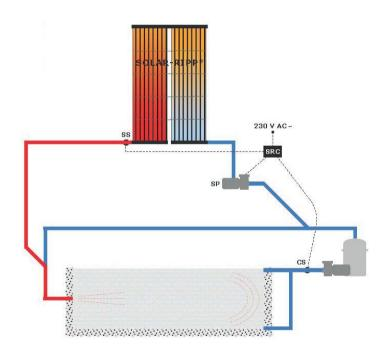
These systems are installed for bigger pools where the complete pool water volume cannot be transferred through the solar absorber by the installed circulation pump alone (limitation of pool pump layout). Here, as it is also the case for other pool heating systems, only a measured part of the pool water is re-routed through the solar absorber and than mixed with the normal circulating return water.
