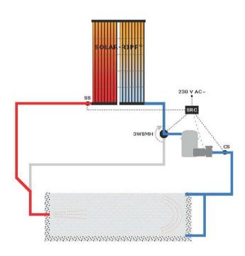
These systems are for smaller to medium sized pools where the installed pump allows for a complete transfer of the water volume through the solar absorber. Depending to the temperature situation, the installed 3-way automatic valves allows for an automatic switch-over between the solar cycle and standard water circulation cycle.
